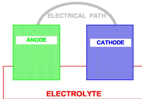
The anode is the part of the metal where corrosion occurs; the anode sacrifices itself to protect the cathode. The anode releases positively charged metal ions into the electrolyte and electrons are left behind in the metal. These electrons flow through the metal to protect the cathode. The cathode is protected because various ions or compounds in the electrolyte consume the electrons.
