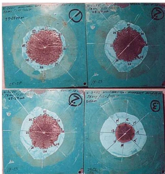
Figure 2. Cathodic disbondment testing.
