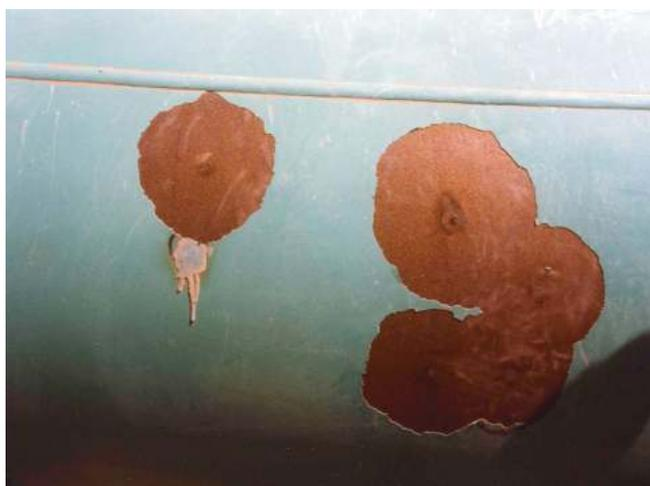
Figure 1. Cathodic disbondment on a pipeline.
