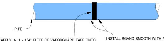
APPLY A 1 - 1/4" PIECE OF VAPORGUARD TAPE ONTO PIPE LEAVING RELEASE LINER ON THE BUTYL
