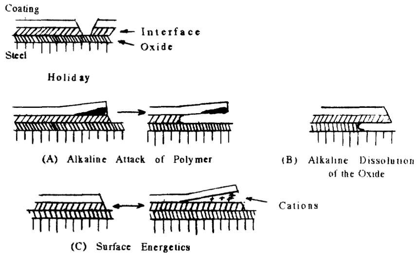
Figure 1 – Proposed mechanisms for cathodic disbonding (after Kendig).
