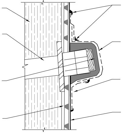
DETAIL SEALANT PW OR LM-95 APPLIED OVER TERMINATION OF FABRIC TAPE AND ONTO BLINDSIDE MEMBRANE -PREPARE FABRIC WITH 650 LT LIQUID ADHESIVE OR CALIFORNIA SEALANT AT A RATE OF 50 - 75 SF/GAL
