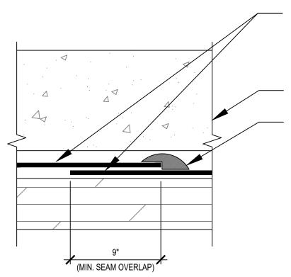
POLYGUARD BALCONY SHEET MEMBRANE SERIES WATERPROOFING OVER POLYGUARD 650 LT LIQUID ADHESIVE OR CALIFORNIA SEALANT APPLIED AT A RATE OF 250 - 300 SF / GAL OR 650 WB LIQUID ADHESIVE APPLIED AT A RATE OF 350 - 400 SF / GAL, INSTALL IN SHINGLE MANNER WITH MINIMUM 9" OVERLAP
