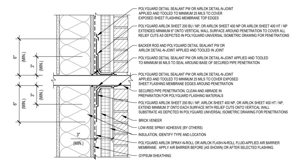
06A STPE SECTION @ FRAMED BACKING WALL / MASONRY VENEER - UNIVERSAL SHEET FLASHING FOR PENETRATIONS
