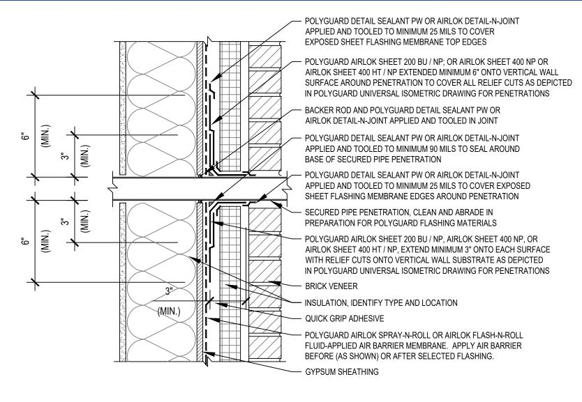
06A STPE SECTION @ FRAMED BACKING WALL / MASONRY VENEER - UNIVERSAL SHEET FLASHING FOR PENETRATIONS
